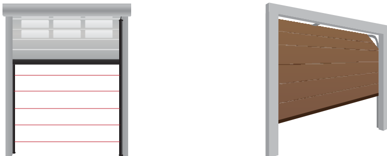
Picture 6. example on rapid doors and sectional doors
